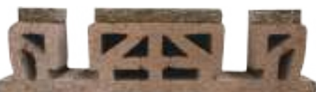
Floor slab S25 + 5 - U=0,60 W/m²K
